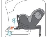
**3.** Put the child seat on the vehicle seat and aim both ISOFIX Connectors (4) to the ISOFIX Anchoring Points 21 in the vehicle seat.
