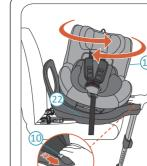
Squeeze the Rotation Release Handle (10) to release the child seat Shell from its locked position. Now vou can rotate the child seat Shell. The child seat Shell has 2 locked positions, forward-facing and rearward-facing. When the child seat Shell is moved to a locked position, it will automatically lock with a click sound. The child seat Shell also has two side intermediate stopping positions (unlocked) so that the child can be put in or take out from the seat easily.
