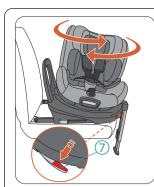
Pull the Rotation Release Handle (7) to release the child seat Shell from its locked position. Now you can rotate the Shell. The Shell has 2 locked positions, forward-facing and rearward-facing. When the Shell is moved to a locked position, it will automatically lock with a click sound and the Rotation Release Button will go back into the Base. The Shell also has two side intermediate stopping positions (unlocked) so that the child can be put in or take out from the seat easily.
