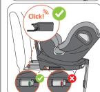
3. Push one ISOFIX Connector to engage it with the ISOFIX Anchoring Point with a click sound. Repeat the action on the other side to engage both ISOFIX Connectors.
