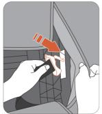
5. Hide the Shoulder Harness and Lap Harness in the side wings of the Shell, behind the cover of the child seat. There's reserved space for them in the side wings of the Shell.
