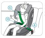
2. Place the Shoulder Belt Section (32) and the Lap Belt Section (33) on the side of the buckle into the Lap Belt Guide 4 of the Base.
